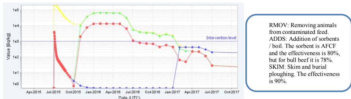
Figure 3: Comparison of the cesium activities of cow's milk in a summer release. Curves in different colors represent cases in which diverse strategies are adopted. The red curve corresponds to taking RMOV between 0-90 days, and then taking ADDS between 90-540 days and SKIM after 90 days. The blue curve corresponds to the action RMOV between 0-540 days. The green curve corresponds to the action RMOV between 0-90 days, and then applying SKIM after 90 days. The yellow curve corresponds to the action "no measure" and is given for comparison
