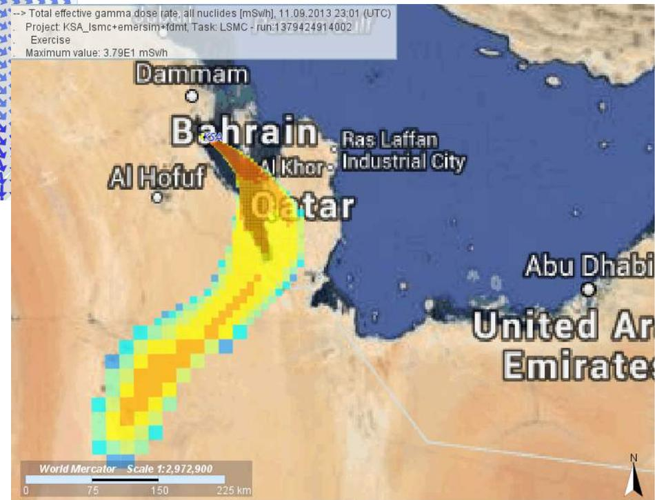
Right: Total effective gamma dose rate, using the NOMADS weather data for a fictive release from a fictive reactor in Saudi-Arabia (JRodos screenshot)
